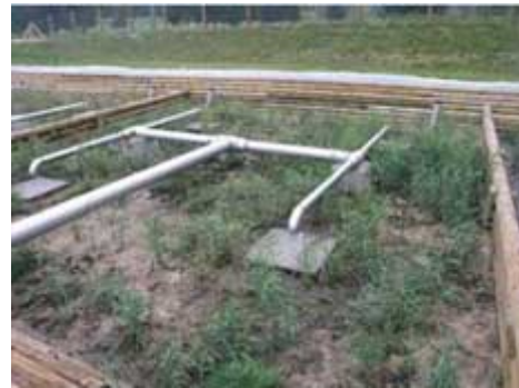
H feeding via an overhead system
