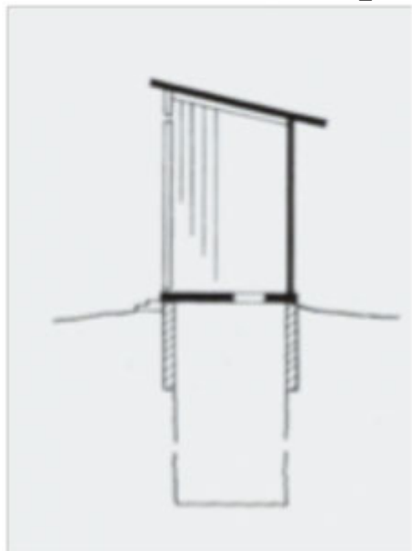
Cross-section of a dry, single-pit latrine
