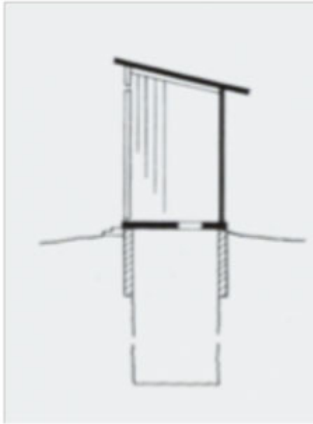
Cross-section of a dry, single-pit latrine
