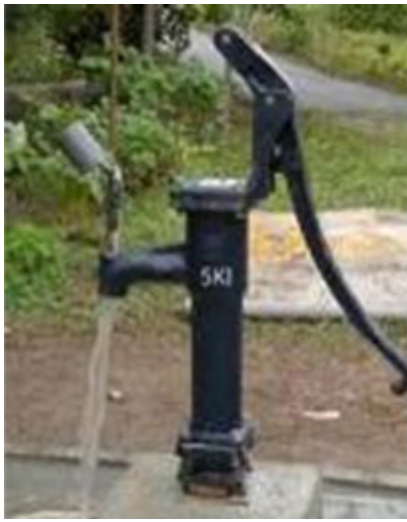
Shallow suction pump designed with UNICEF_Malaysia's help
