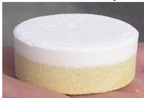
This product is marketed in the form of two-layer double-sided tablets that successively carry out a double action of clarifying and disinfecting water. The first is made up of a coagulant, iron sulphate, and the second of sodium dichloroisocyanurate for chlorinating and disinfecting the water.
